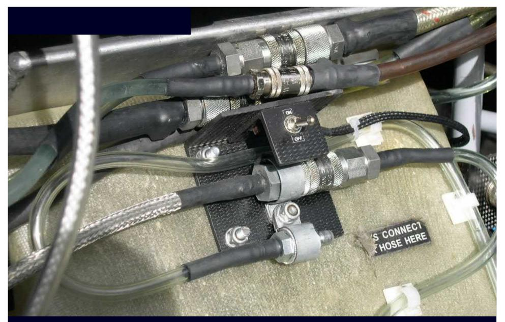
At every refilling, all quick couplings have to be open and gasoline drops onto the electric switch.
