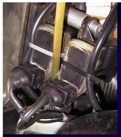
Modified by owner: original connectors and e-boxes at centerline of vibrations
