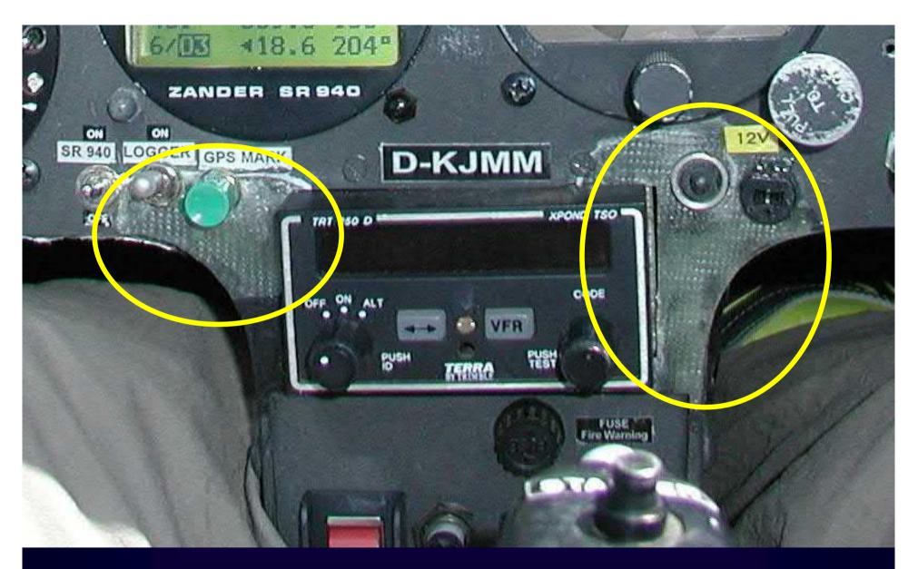
Result of vibrations: the instrument panel broke on both weaker sides.
