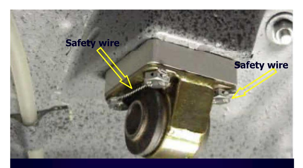
SHK Spindle support: Until September 2000, the (4) screws of the spindle drive were not secured. One fell away!
