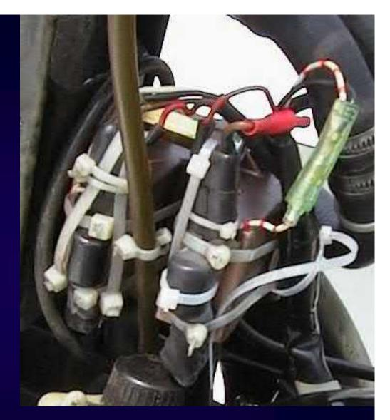
Modified by owner: no connectors and e-boxes at centerline of vibrations
