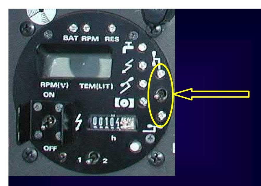
This 1 € switch failed, impossible to retract the engine!
