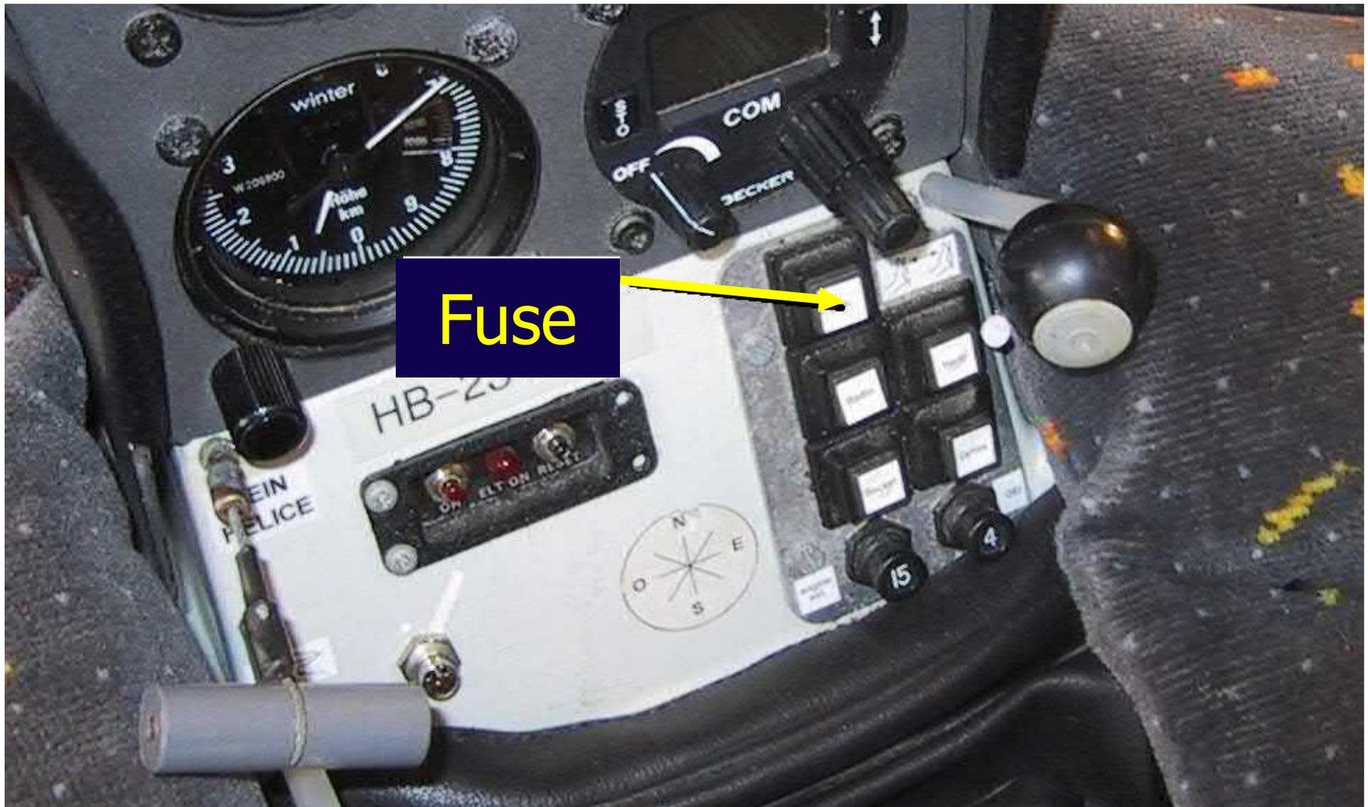
DG 800: the same fuse is used for charging in flight and on the ground: no more charging possible. Engine may not move!
