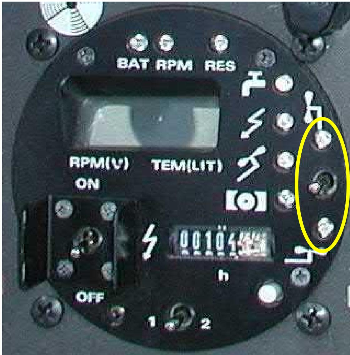
This 1 € switch failed, impossible to retract the engine!
