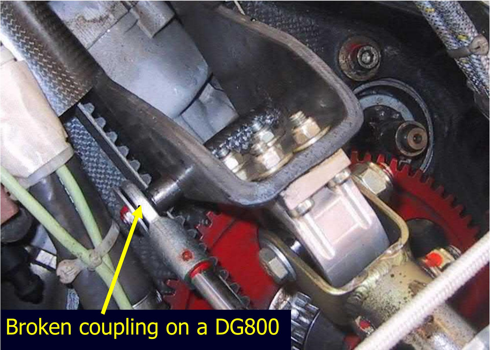
Broken coupling on a DG800
