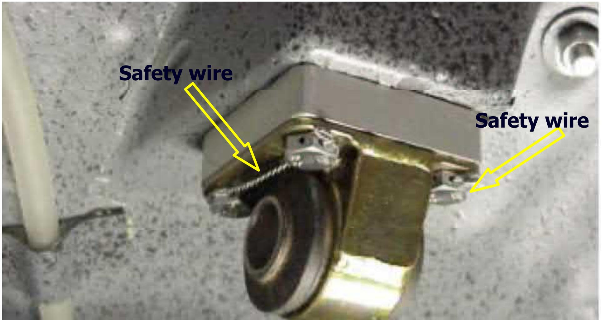
**SHK Spindle support: Until September 2000, the (4) screws of the spindle drive were not secured. One fell away!**
