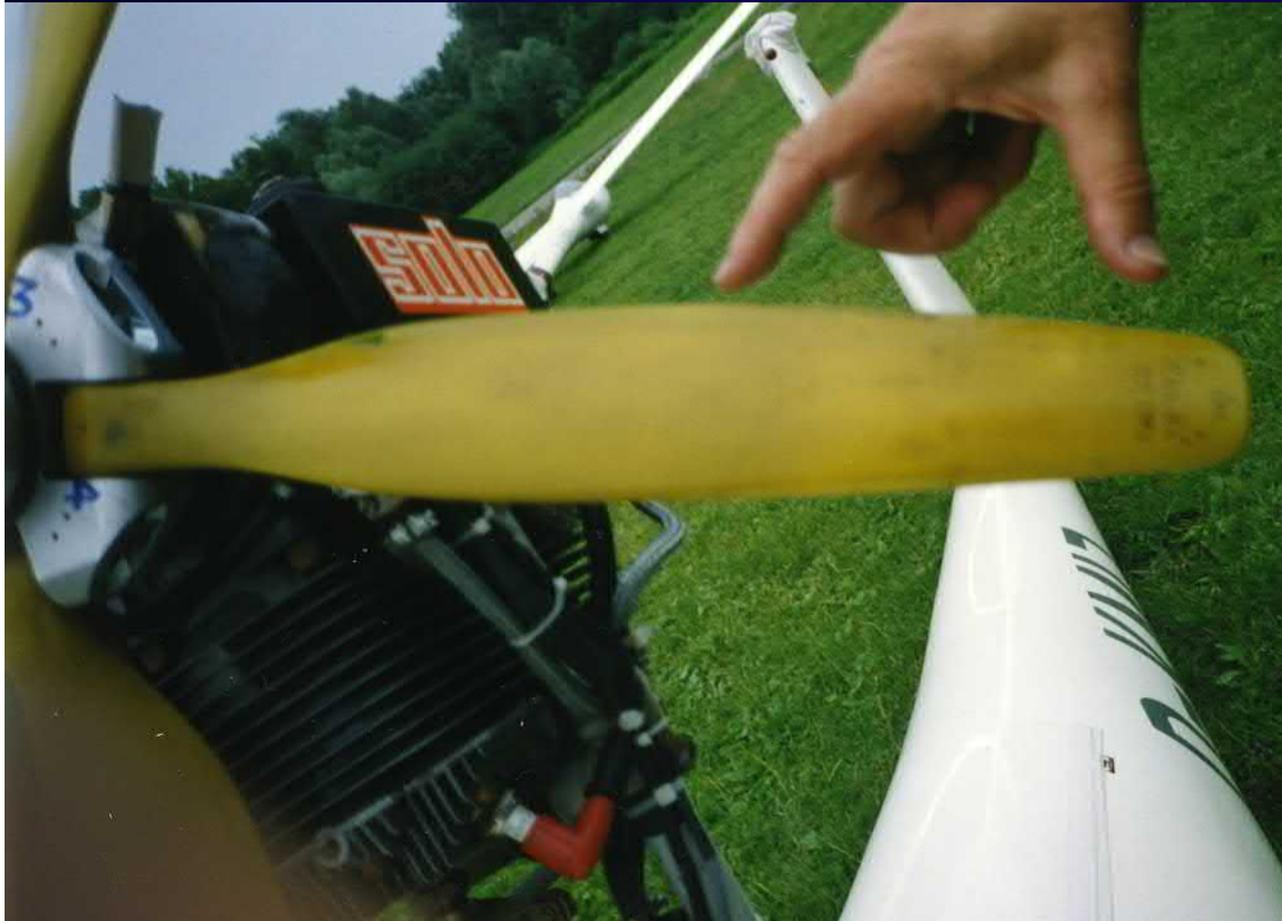
First engine, first problem: One blade is self desintegrating because of speed and vibration (1986)
