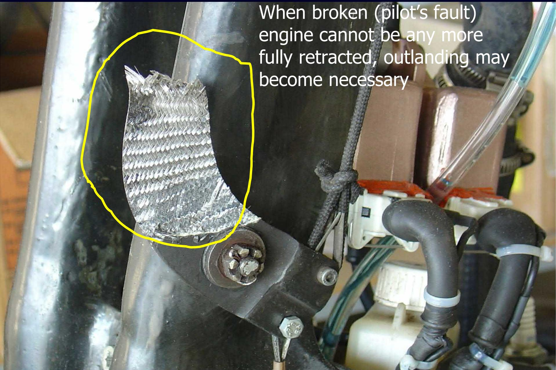
When broken (pilot's fault)
