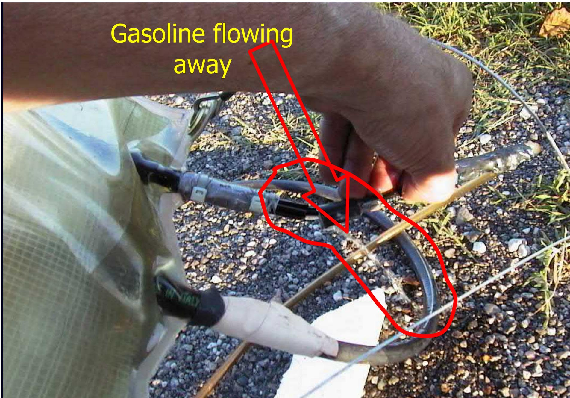
This vent pipe connection is badly leaking
