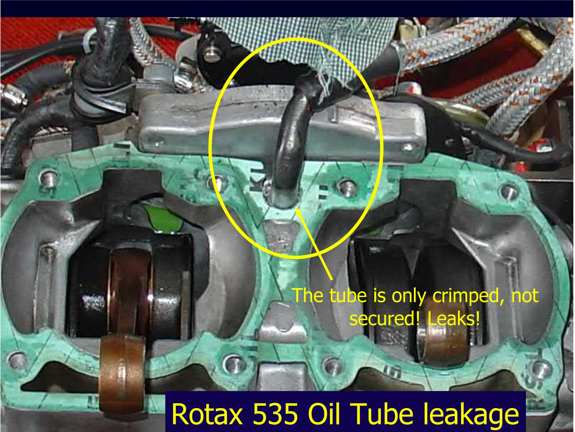
The tube is only crimped, not secured! Leaks!
